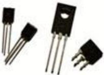
Semiconductor devices used to amplify electrical signals (in stereos, radios, etc.) or to act like a light switch turning the flow of electricity on and off.
